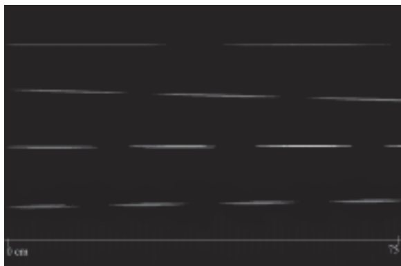
Figure 2. A photograph of the optical rotation of laser light as it propagates through a sucrose solution. The wavelengths seen here are 632 nm (from a HeNe laser), 514 nm, 488 nm, and 457 nm (from an argon ion laser).
