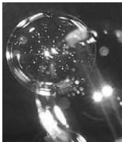
Figure 2. Double bubbles: when a smaller bubble contacts a larger bubble, the higher pressure of the smaller bubble causes it to protrude into the larger one.
