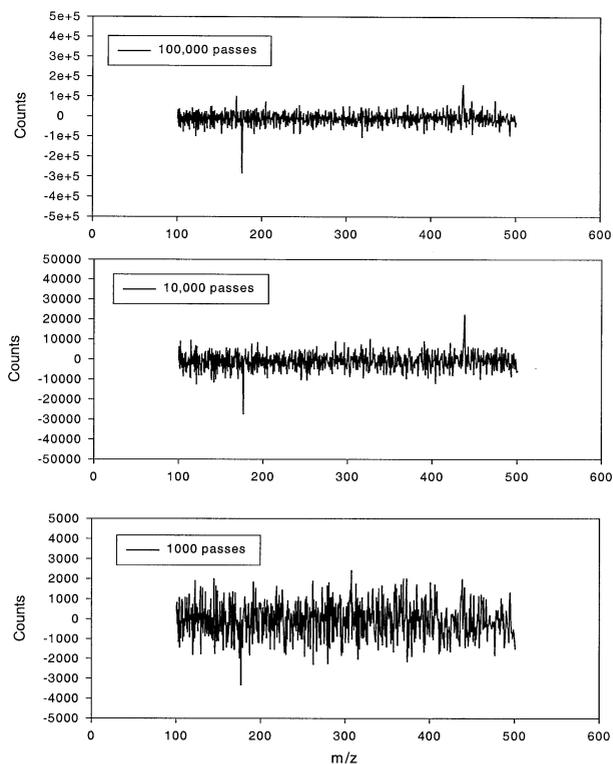
**Figure 4.** Baseline signal between 100 and 500  $a\mu$  for three different acquisition times. One thousand passes correspond to 0.8191 s. The data was acquired in HT-TOFMS mode for a sequence length of 8191 (13 bits) with a modulation voltage of 30 V.
