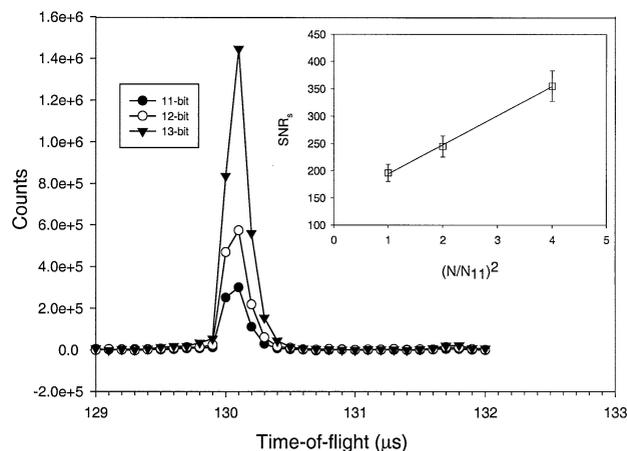
**Figure 5.** Peak height intensities of a 100  $\mu\text{M}$  solution of reserpine in 50:50 methanol:water (1 mM acetic acid) modulated by different pseudo-random sequences. The insert shows the improvement in SNR as a function of the relative increase in the sequence length compared to a 11-bit sequence ( $N/N_{11}$ ).
