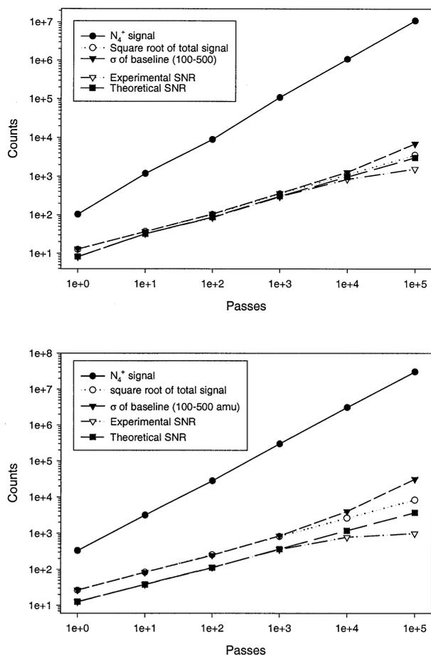
**Figure 3.** Simplex signal-to-noise ratio  $SNR_S$  in a nitrogen corona discharge. (a)  $SNR_S$  for a monomolecular ion beam of  $N_4^+$  and (b) an ion beam with all nitrogen ionic species.
