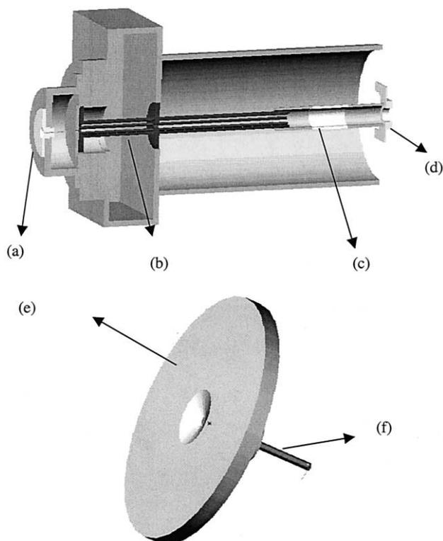
**Figure 1.** Schematic of the HT-TOFMS spectrometer. Top: first three differentially pumped regions of the instrument: (a) Interface, (b) octopole, (c) cylindrical lenses, (d) ion beam modulator. Bottom: Electro spray interface, (e) ground plate, (f) nozzle.
