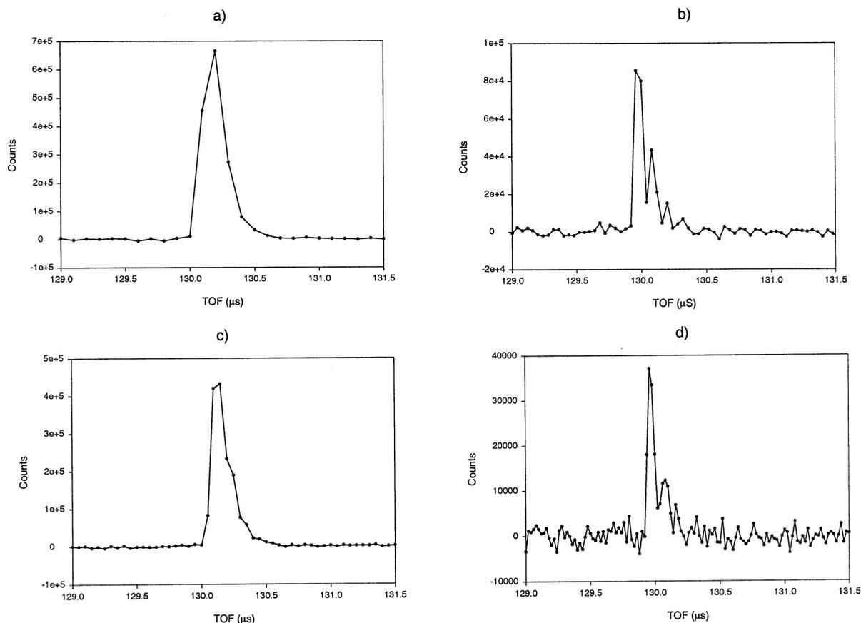
**Figure 6.** Effect of the modulation and acquisition time bins on the resolution under a 12 bit pseudo-random sequence. (a) 100 ns modulation bin, 100 ns acquisition bin; (b) 40 ns modulation bin, 40 ns acquisition bin; (c) 100 ns modulation bin, 50 ns acquisition bin; and (d) 40 ns modulation bin, 20 ns acquisition bin. (50,000 passes).
