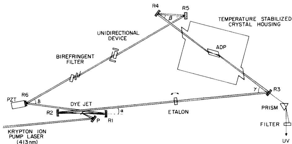
Fig. 1. Schematic of the coumarin ring laser: P = pump mirror;  $\alpha \approx 4^\circ$ ;  $\beta \approx 25^\circ$ ;  $\gamma \approx 34^\circ$ ;  $\delta \approx 42^\circ$ ; mirrors  $R_1 = R_2 = 5 \text{ cm}$ ,  $R_3 = R_4 = 50 \text{ cm}$ ,  $R_5 = R_6 = \infty$ ; and PZT = piezoelectric translator.
