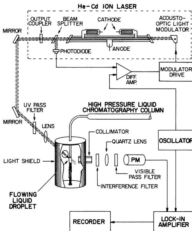
acousto-optic light modulator, reduces the root-mean-square noise of the laser and ensures that the laser power is directly proportional to the applied oscillator voltage. The signal from the photomultiplier which is in phase with the oscillator is detected by a lock-in amplifier, whose output drives a stripchart recorder.
